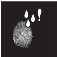
Fingerprint too dark. Dry finger (shake hand in air) or apply less pressure on fingerprint sensor.
