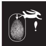
Fingerprint entry too fast. Swipe finger slower and longer over fingerprint sensor.
